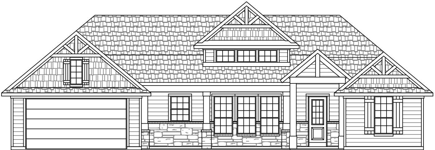
ELEVATION "C" ALL SIDING W/ PORCH MASONRY
